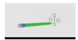
Draw a small dot in each of the four holes then make an "X" by connecting the dots.
